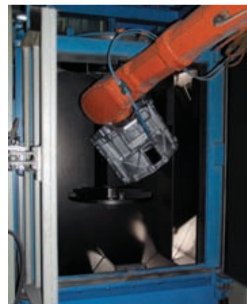
Integrated deburring of aluminium die-cast parts
