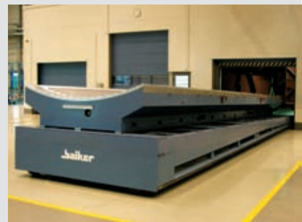
peen forming system for Airbus to automatically process aircraft skin plates
