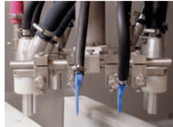
Inside view of blast chamber showing the six reciprocating nozzles for blasting rinsing and blow off
