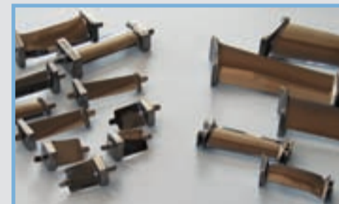
Typical turbine blades - processed in the new high-speed vibrators
