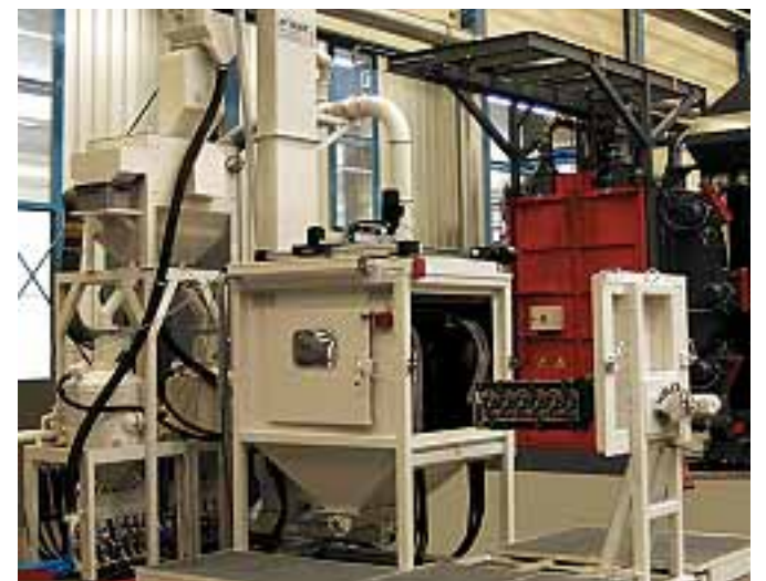
STD 1400 PS-So removes casting sand deposits from cylinder head blocks
