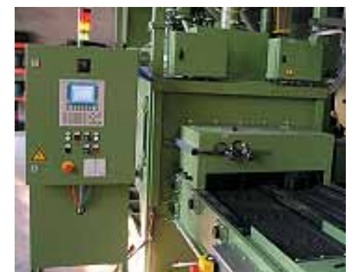
Two parts conveyors ensure the springs are shot blasted on both sides
