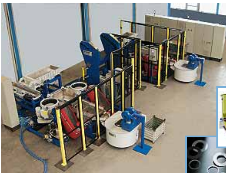
Efficient tandem centrifugal disc finishing systems with shared separation and drying units
