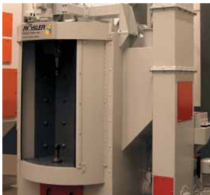
Oscillating chamber shot blast system: simultaneous shot blasting and loading/unloading
