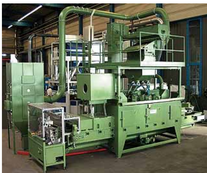
RBD system shot peens 1.5 million disk springs a year
