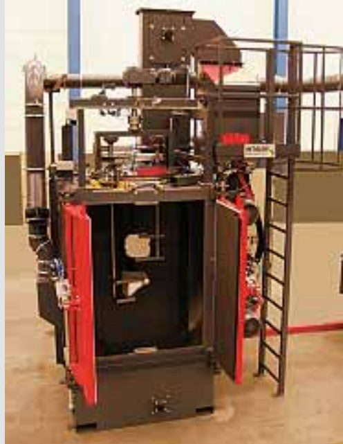
Aluminum diecast parts are deflashed in seconds
