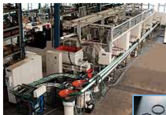
Eight interconnected centrifugal disc machines provide a high level of automation
