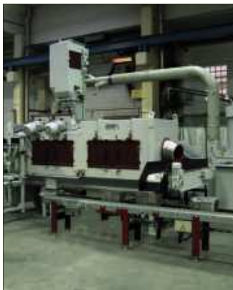
The balancing weights are transported continuously in bins to the continuous tumble belt machine for shotblasting.
