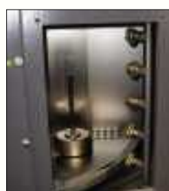
After passing through the blow-off section, the components are almost dust free. This prevents media carryover into the loading and unloading area.
