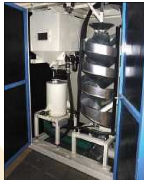
An important aspect of shot peening is precise classification of the shot peening media. This picture shows the single spiral separator for removing unusable media.
