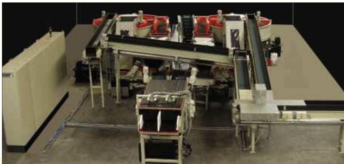
Two Rotomatic R 370/12 SE's in a tandem configuration. Front centre: The separation and passivation machine is used by both Rotomatics.
