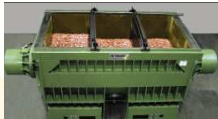
"New tub vibrator "TS/D" with adjustable imbalance weights.
