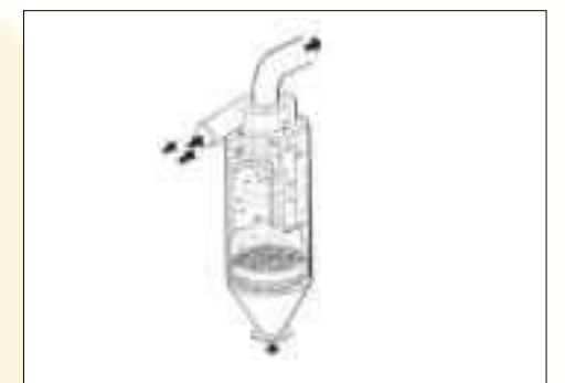
In a cyclone separator, dust and light particles are removed.
