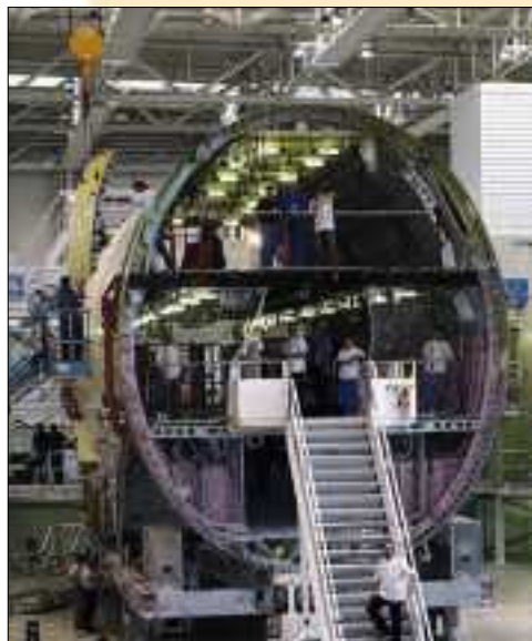
The raw materials used in the new Super Airbus are of particular interest. The structural components of the fuselage are shot peened by Rösler shot blasting technology, making them distortion-proof and resistant to fatigue cracks.
