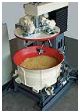
A space-saving machine concept with versatile technology: the R1-1/4 SSA-C compact drag finishing system
