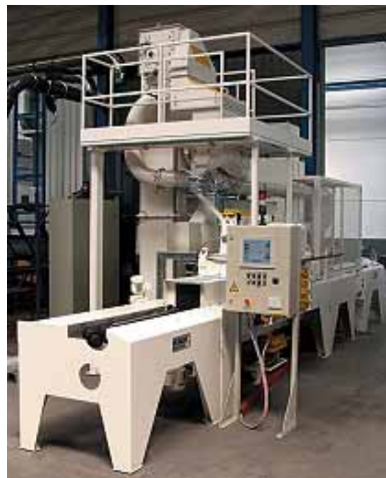
The RDR 100 peens the surfaces of manganese steel stabilizers
