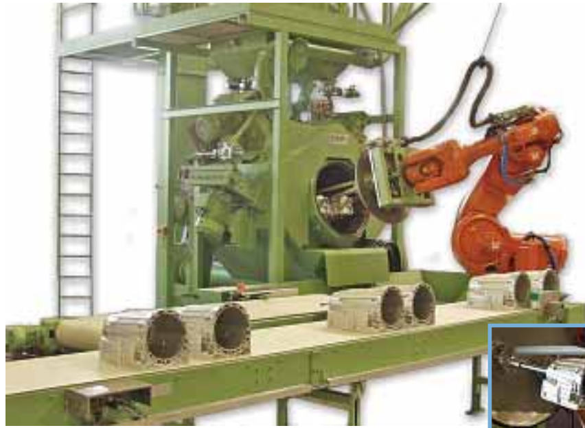
Rösler developed this highly efficient processing system for an automobile manufacturer to deburr and surface finish transmission housings.
