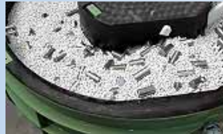
The surfaces of bearing rollers are polished in a rotary vibratory bowl by the Keramo-Finish® process
