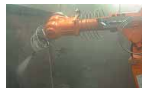
The Rösler high-pressure wet blast system cleans the component at a pressure of 4000 bar
