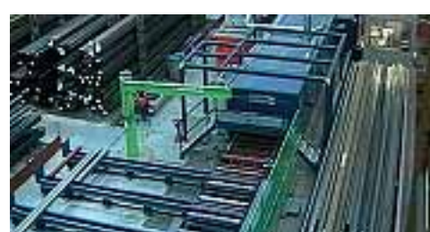
Over 100,000 tons of steel pass through the CWT preservation line per year, where they are shot blasted and then coated with a welding primer layer
