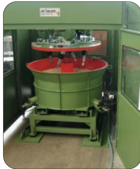
The „Mini“-drag-finishing machine R 1-1/4 SSA-L makes the advantages of drag-finishing available to a larger market
