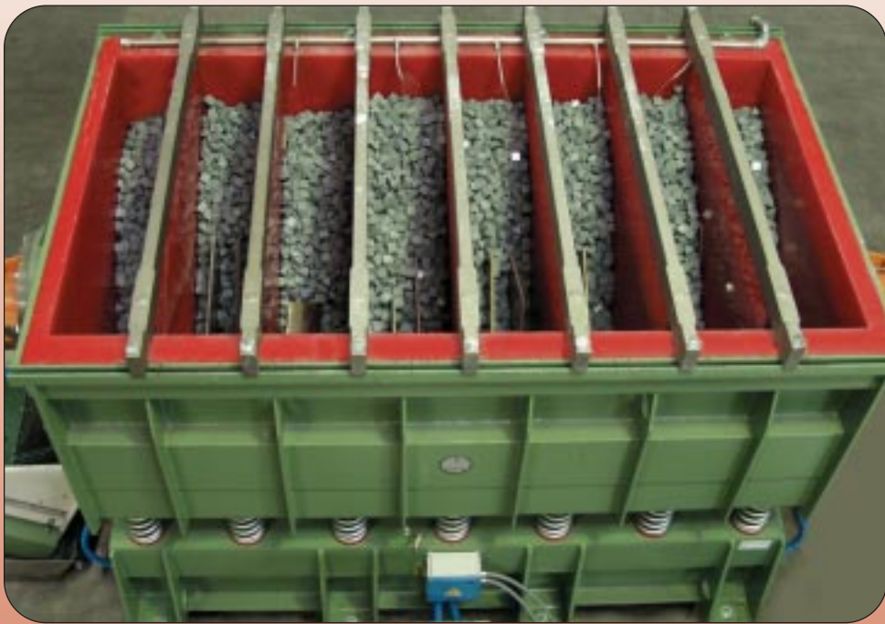
For emptying, the trough vibrator has a side mounted unload door, the chips are transported to a magazine by a conveyor belt.
